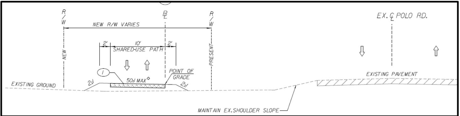
**Exhibit C: Shared-Use Path Typical Section (Bicycle / Pedestrian Specific Project; Non-Capacity Project)**
